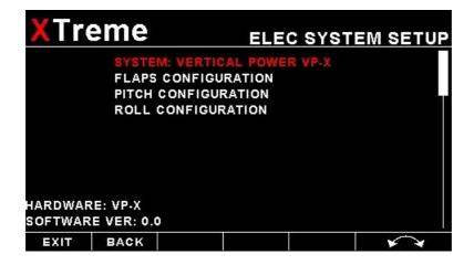
The electrical system setup menu option allows the pilot to select what electrical system/ECB (Electronic Circuit Breaker) is attached to the XTreme EFIS. The XTreme supports the Vertical Power VP-X range of electrical systems/ECBs.
