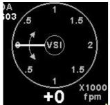
This displays the VSI as a traditional VSI indicator. The scale and units can be configured in the "VSI SETUP" menu.
