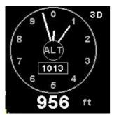
This displays the altitude as a traditional 3 needle analog altimeter. A digital readout of the altitude value is also displayed below the dial. The altitude parameters can be configured in the "ALTITUDE SETUP" menu.
