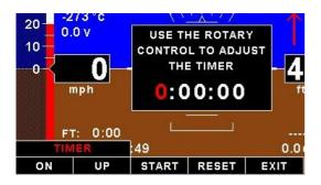
Select this menu option to configure the timer. Use the rotary control to adjust the timers reset value. Press the "UP/DOWN" soft key to select whether the timer must count up or down, the "START/STOP" soft key to start or stop the timer and the "ON/OFF" soft key to enable or disable the timer.
