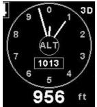
This displays the altitude as a traditional 3 needle analog altimeter. A digital readout of the altitude value is also displayed below the dial. The altitude parameters can be configured in the "ALTITUDE SETUP" menu.
