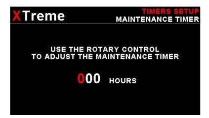
These timers allow you to keep track of engine maintenance interval. Set the timer when you have serviced your engine. A typical time might be 50 hours. This function allows you to set an engine maintenance timer. This timer is set in engine hours and it will count down to zero when the engine RPM is greater then the "HOBBS MINIMUM RPM". A good use for this function is to set the hours until your next spark plug change or engine inspection. Use the rotary control to change the value.
