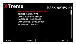
Select this menu option to mark a waypoint. The latitude, longitude and altitude are automatically set based on the current location. Enter a short name and long name for the waypoint so you can easily identify it. Press save once you have finished editing and to save the waypoint to the waypoint.ewd file.
