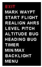
Press the rotary control when the EFIS screen is displayed to access the EFIS quick select menu
