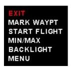
Press the rotary control when the GPS screen is shown to access the GPS quick select menu.
