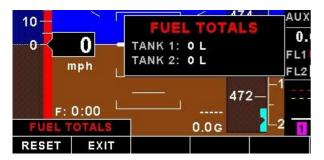
Select this menu option to display the fuel totals. Press the "RESET" soft key to reset the totalisers to zero. Press the "EXIT" soft key when done.
