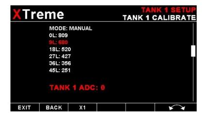
You may want to set individual calibration points manually. For example you may find that your fuel level is over reading at a specific fuel level. Correcting the tank level reading for this area can be simply done by adjusting the calibration point. You can do this by moving the float level with your hands to the desired position and then performing the calibration as outlined above, or you can use the manual option.
