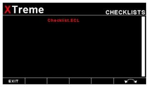
Copy the created file (.ECL extension) to the checklst directory on the SD card when you are complete. The checklist file can be loaded by pressing the rotary control and selecting "CHECKLISTS". A window containing all the files with the .ECL extension will shown. Select the checklist you require. The number of checklists that can be stored and displayed depends on the size of the SD card.
