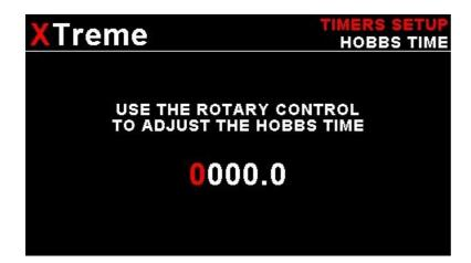
This function allows you to set the engine Hobbs meter to any value. Typically, you would use this function to set the Hobbs meter to the current known engine time. Use the rotary control to change the value. Press the rotary control to accept and exit the menu option. If the Hobbs code is set to another value beside zero, then the pilot will be prompted to enter the Hobbs access code before allowing him to change the Hobbs time. This feature is useful for charted and flying school planes.
