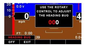
Use the rotary control to adjust the heading bug. Press the "ON/OFF" soft key to enable or disable the heading bug.
