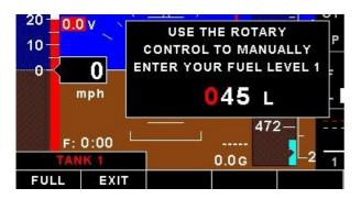
Select this menu option to refill a calculated fuel tank. Press the *"FULL"* soft key for a quick fill to the full reading in the tank setup menu. Press the *"EXIT"* soft key when done.
