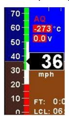
This is located to the left of the EFIS display. The Vso (Min safe speed, landing), Vs1 (Min safe speed, normal), Vfe (Max flap speed), Vno(Max maneuvering speed) and Vne (Max exceed speed) can be configured in the "AIRSPEED SETUP" menu.
