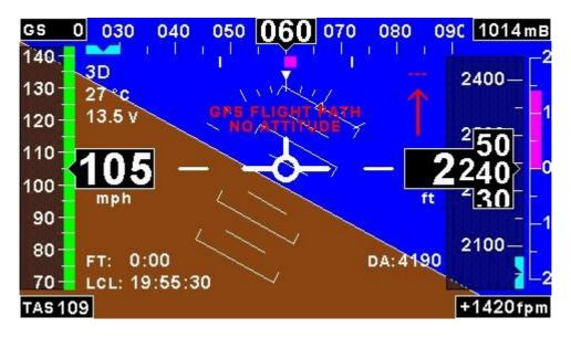
The GPS Flight path feature uses a method to calculate bank and pitch angles from information obtained from the internal GPS receiver. This is no means a replacement for a real gyro based AHRS unit but is more intended as a informative / simulated display of the horizon.
