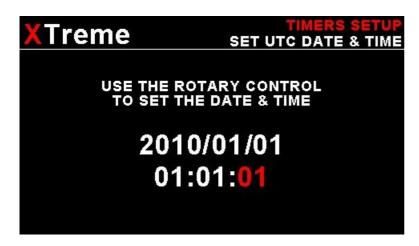
Use the rotary control to set the UTC date & time in the internal RTC.
