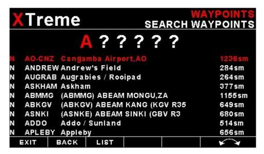
Use the rotary control to enter the search string for the short name. Once the required waypoint is visible in the list press the "LIST" softkey. Use the rotary control to scroll up and down the list. Press the rotary control to select the required waypoint.
