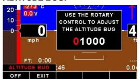
Use the rotary control to adjust the altitude bug. Press the "ON/OFF" soft key to enable or disable the altitude bug icon.
