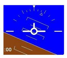
The horizon line separates the ground from the sky just like a conventional gyro based artificial horizon. The ground color can be selected to be shown in green or brown.
