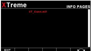
The graphic information file can then be loaded by pressing the rotary control and selecting "INFO PAGES". A window containing all the files with the .MIF extension is shown. Select the desired information page. The number of information pages that can be stored and displayed depends on the size of the SD card.
