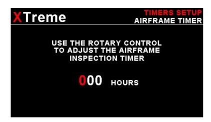
This timer operates similar to the engine maintenance timer but is based on flight time. You might use it to schedule thorough airframe checks at intervals, perhaps every 25 or 50 hours.
