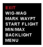
Press the rotary control when the electrical system screen is shown to access the electrical system guick select menu.
