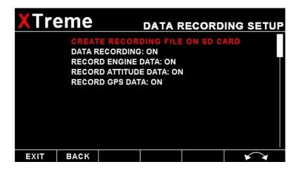
The XTreme has the ability to act as a black box recorder recording flight data directly onto an inserted SD card for later playback and investigation using the MGL Avionics Enigma Black Box viewer program. See the Enigma Black box viewer documents for further information. The Black box viewer can also convert the data into other file formats such as:
