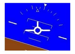
Select whether the bank indicator markings are "MOVING" or are "FIXED" (default) The "FIXED" bank indicator has an clear arrow which moves to stay perpendicular with the horizon, the "MOVING" bank indicator rotates the scale around a stationary arrow.
