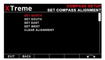
The purpose of this function is to cancel out the remaining errors on the main cardinal headings after a deviation compensation calibration has been done.
