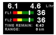
3.12.4.3 Single fuel flow and dual fuel level senders (dual tank)
