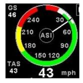
This displays the airspeed as a traditional analog airspeed indicator. A digital readout of the airspeed value is also displayed below the dial. The Vso (min safe speed, landing), Vs1 (min safe speed, normal), Vfe (max flap speed), Vno(max maneuvering speed) and Vne (max exceed speed) can be configured in the "AIRSPEED SETUP" menu.
