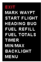
Press the rotary control when the VFR screen is displayed to access the VFR quick select menu.
