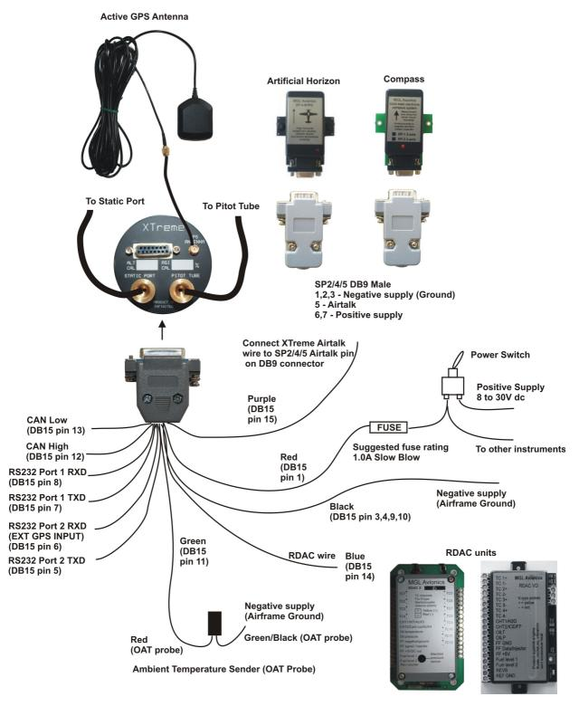
The use of an external 1A fuse is recommended. Connect the supply terminals to your aircrafts power supply. The XTreme can be used on both 12V and 24V without the use of any pre-regulators. Ensure that the supply voltage will not drop below 8V during operation as this may result in incorrect readings.
