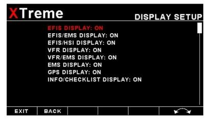
The display setup menu option allows the pilot to select if certain display screens must be shown or not when toggling through the displays using the left or right most soft keys.
