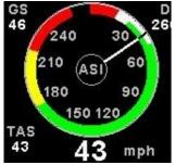
This displays the airspeed as a traditional analog airspeed indicator. A digital readout of the airspeed value is also displayed below the dial. The Vso (min safe speed, landing), Vs1 (min safe speed, normal), Vfe (max flap speed), Vno(max maneuvering speed) and Vne (max exceed speed) can be configured in the "AIRSPEED SETUP" menu.
