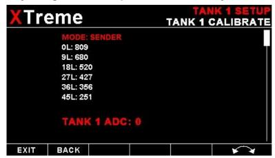
Select "SENDER" for the "MODE" menu item. Once you have installed a fuel level sender into your tank, make sure the float can travel all the way from empty to full position without hindrance of any kind. The calibration procedure should be carried out with your aircraft in flight attitude. This means you need to lift the tail if you have a tail-dragger or lift the nose wheel if you have a weightshift trike.
