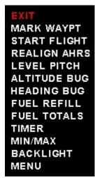
Press the rotary control when the EFIS/EMS screen is displayed to access the quick select menu.
