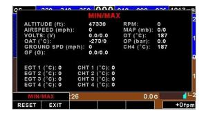
Select this menu option to display the maximum and minimum captured values. Press the "RESET" soft key to reset the min/max values to the current values.
